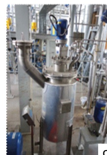
Fig. 3 Adaptation and development of continuous flow installation for pilot scale HTL experiments at 2 kg/h (GIG-NRI): (a) continuous flow installation at GIG-NRI's Clean Coal Technology Centre; (b) constructing of HTL reactor; (c) constructing of slurry pumping system.
