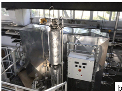
Fig. 3 Adaptation and development of continuous flow installation for pilot scale HTL experiments at 2 kg/h (GIG-NRI): (a) continuous flow installation at GIG-NRI's Clean Coal Technology Centre; (b) constructing of HTL reactor; (c) constructing of slurry pumping system.
