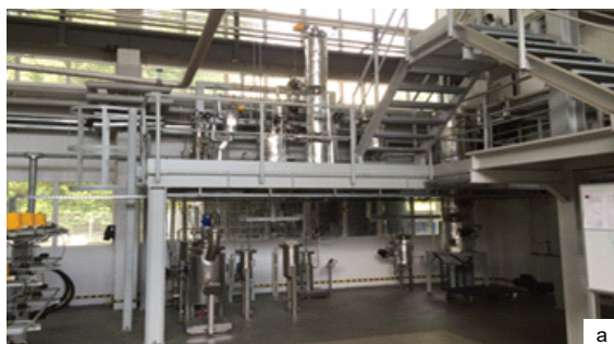
Fig. 3 Adaptation and development of continuous flow installation for pilot scale HTL experiments at 2 kg/h (GIG-NRI): (a) continuous flow installation at GIG-NRI's Clean Coal Technology Centre; (b) constructing of HTL reactor; (c) constructing of slurry pumping system.
